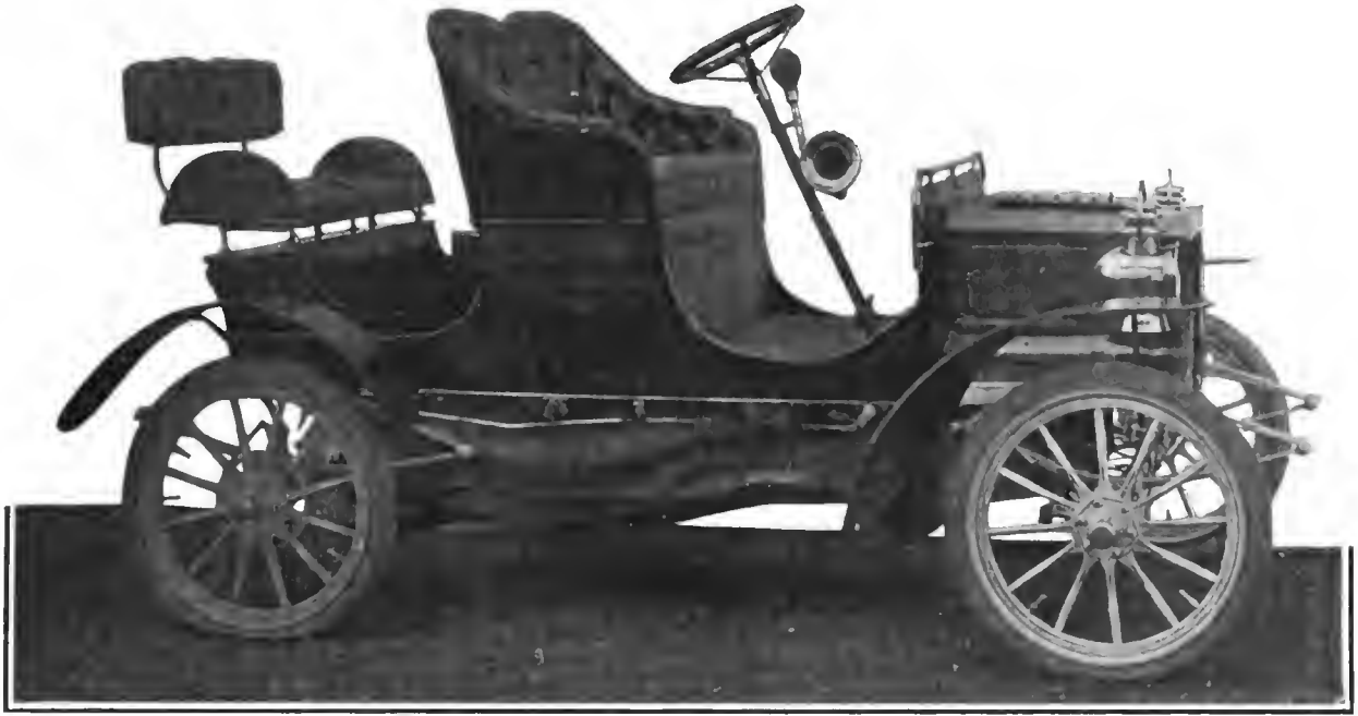
REO 8-HORSEPOWER RUNABOUT FOR 1906, WITH REAR FOLDING SEAT OPEN FOR EXTRA PASSENGERS.
